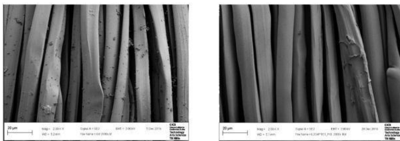
Fig. 1 - Artificially aged and soiled silk fibres (left) and aged silk fibres after cleaning with 1064 nm laser 5 pulses and 1 J/cm 2 (right).
