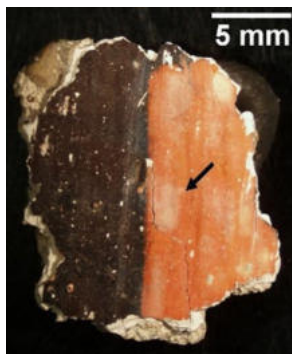
Figure 1. Darkened red lead paint sample after irradiation by a CW top-hat Nd:YAG laser (red part on the right) at 1000 kW m -2 . The lighter stains designated by an arrow are due to gypsum. Cracks were present before the treatment.
